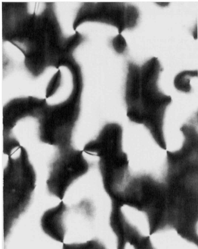
Figure 5. A laser-aligned area as viewed through a single polarizer with the transmission axis at 45^\circ to the rubbing axis. The exposure was for 3 min at 8 \text{ W/cm}^2 and clearly demonstrates domains with directors pointing clockwise and counter-clockwise from the initial alignment direction.
